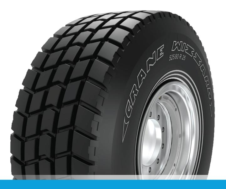
The new Crane Wizzard™ non-directional tire line supports three popular sizes (525/80R 25, 445/95R 25 and 385/95R 25). Designed with end-user feedback, Crane Wizzard tires complement the steel and aluminum wheels OTR supplies to the crane market with a "system solution," offering a better value ratio (function vs. cost). Tires are FMVSS 119 and EU/ECE compliant, with E-marks.
