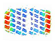
Wide contact patch coupled with unique design means an NDX tire maintains an optimal profile, even under heavy loads (as confirmed by deflection measurements).
