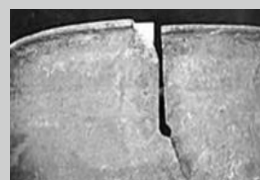
Cracked Wheel Flange
